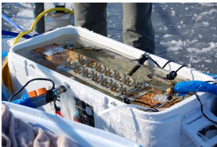
Figure 1. Incubation of quartz tubes for assessing photochemical changes in seawater samples. Time series exposures were 0, 24, 48, and 72 h. Waters from two sites were exposed for 96 h. Water temperatures in the flow-through system were maintained above freezing ( 2 \pm 1 °C Mean \pm
