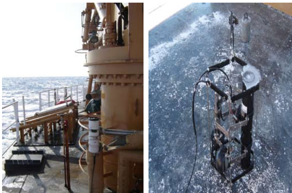
Figure 1. The optical instruments. The left figure shows the surface unit PRR-810 fixed on the left side of stern. It was mounted on the right side of stern if the sunlight came from the starboard. The right figure shows the PRR-800 (right) and MCTD (left), which is mounted on the same frame for profiling. The frame is specially designed to keep the instruments' balance in water and not to shade the PRR-800. Two weight balls were fixed on the frame to increase the vertical stability of the underwater unit. Another weight cylinder (shown on right-up corner in the right figure) was hung on the frame with a gray rope for the same purpose.
