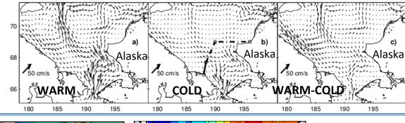
As an additional result of these studies we obtained two MDOTs for the Pacific <sup>70</sup> AO (a,b), which may be used as a reference SSH for assimilation of satellite altimetry observations (c)
