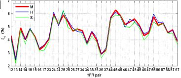
Relative reduction of the errors in estimation of the mass (M), Heat (H) and salt (S) transports for various pairs of the HFRs. Number labeling HFR pairs correspond to location HFR.
