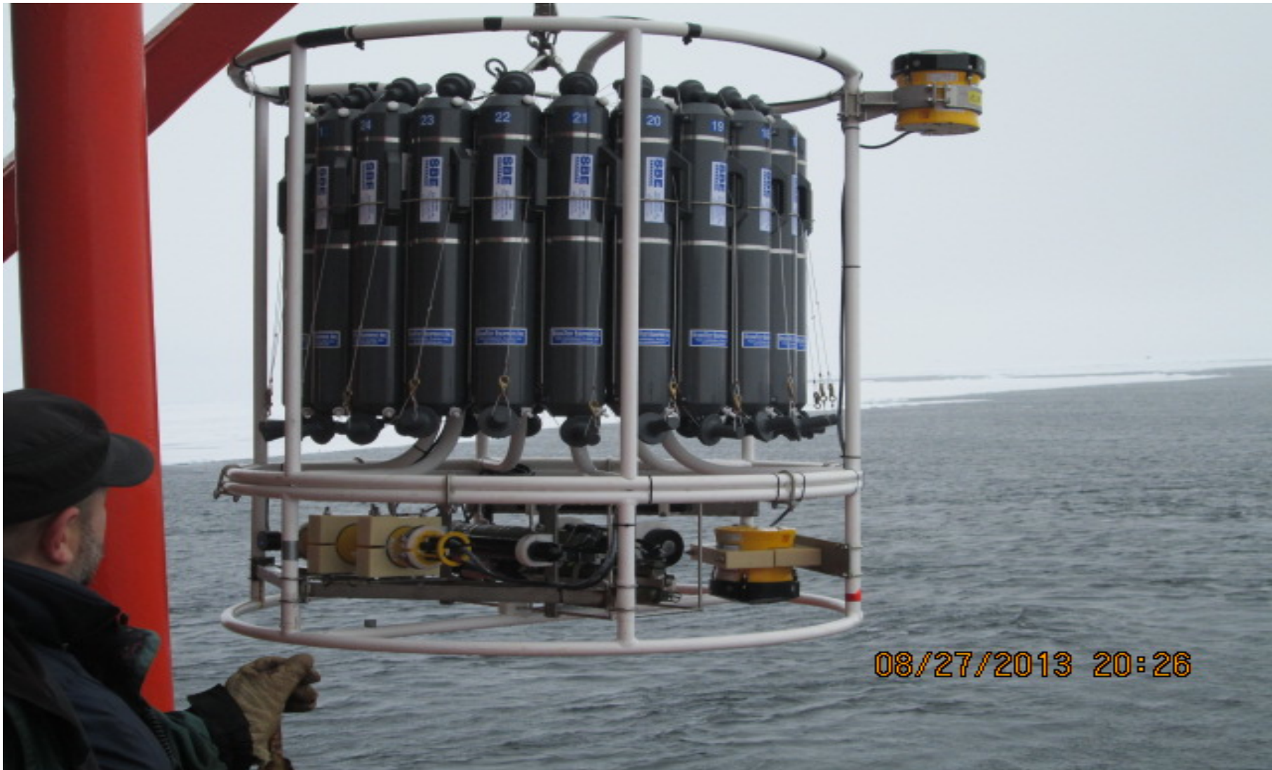
24 bottle (10 L) rosette, CTD with dual conductivity & temperature sensors, dual O 2 sensors, SUNA NO 3 sensor, WET Labs ECO FLNTU (Chl F & turbidity), C-star (beam attenuation), ADCP, and altimeter
